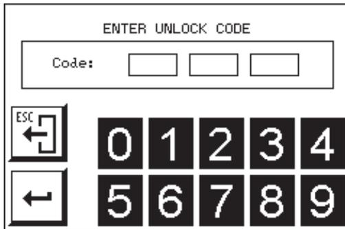
Enter the pin unlock code (PUK) supplied upon purchasing the equipment and press .
