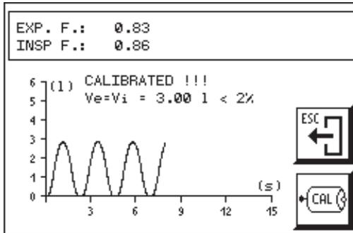
**6** Once calibrated, exit the Calibration Program and access the Spirometry program to begin the tests.
