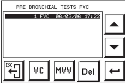
Using keys **VC** and **MVV**, the VC and MVV tests can be seen and saved in PRE mode.
