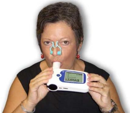
**4** Press the
